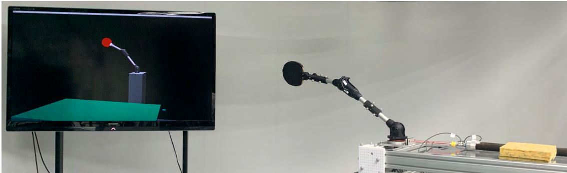
Figure 2.12: Our muscle-based robotic arm is a testbed for Learning for Control. While it offers unique possibilities in terms of high accelerations, extreme speeds and variable stiffness actuation, classical control methods are known to struggle with these abilities.
