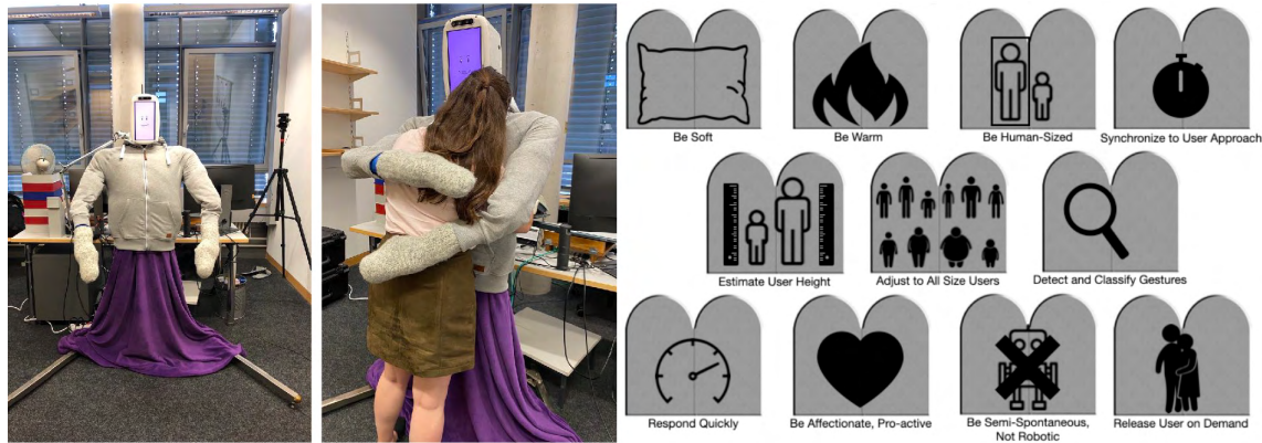
Figure 3.21: We designed, built, and evaluated a series of autonomous hugging robots. Left: HuggieBot 2.0 [647] ready for a hug. This custom human-sized hugging robot has two padded arms, an inflated torso, and a face screen mounted to a rigid frame. Center: HuggieBot 2.0 hugging a user. A camera above the screen visually senses the user at the start of the interaction, and torque sensors on the shoulder flexion and elbow flexion joints are used to embrace the user with a comfortable pressure. Right: The eleven hugging design guidelines that have been validated through this project.
