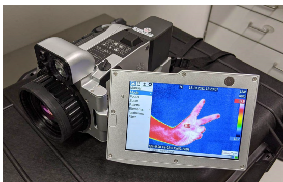
Figure 6.12: Infrared camera creating a temperature map of a human hand.
