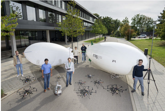
Figure 4.11: Flying motion capture of humans and animals presents many challenges: tracking, calibration, and autonomous control to name a few. To enable long flight times and quiet operation, we are developing a 3D motion capture system based on lighter-than-air vehicles. Such blimps present new challenges beyond existing fixed rotor vehicles since they are deformable and susceptible to wind.
