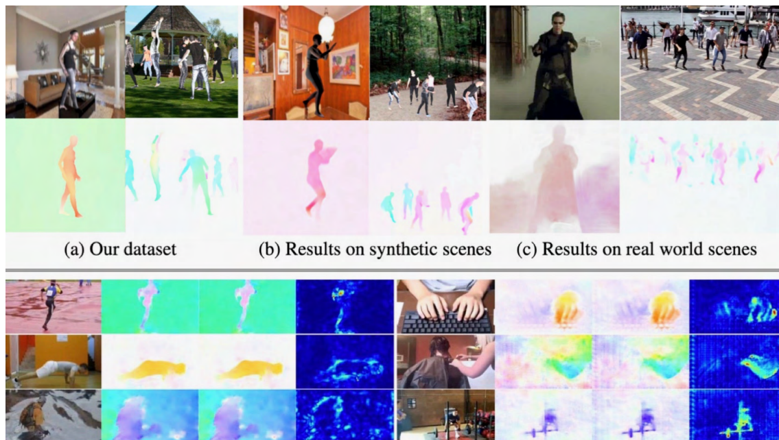
Figure 4.37: (Top) We learn human flow [865],[762] from synthetically generated flow fields and find that this generalizes to real videos of human movement. (Bottom) We fine tune an optical flow algorithm to produce flow that improves action recognition [871]. (Left columns) SpyNet. (Right columns) FlowNet. In each set, left to right: first image in sequence, original flow, flow when trained on action recognition, differences in the flow are focused on the human action.
