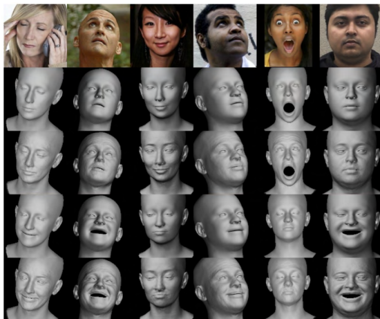
Figure 4.4: DECA [752] is trained to regress face shape and animatable details from in-the-wild images. From top to bottom: Input image, coarse 3D shape reconstruction, detailed shape reconstruction, animation of the coarse shape, predicted details for the animated shape.
