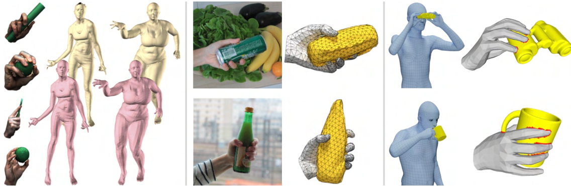
Figure 4.19: (Left) We use a dataset of 3D hand scans to learn MANO, a statistical model of 3D hand shape. We combine MANO with our SMPL body model to build the holistic SMPL+H model. We register SMPL+H (pink) to 4D scans (white); the results look natural even for missing data or finger webbing in scans. (Middle) We train ObMan, a deep network with a MANO layer, to estimate 3D hand and object meshes from an RGB image of grasping, while encouraging contact and discouraging penetrations. (Right) We capture GRAB, a dataset of real whole-body grasps (blue, yellow), i.e. of people interacting with objects using their body, hands and face. We use GRAB to train GrabNet, a network that generates grasping hands (gray) for unseen objects (yellow).
