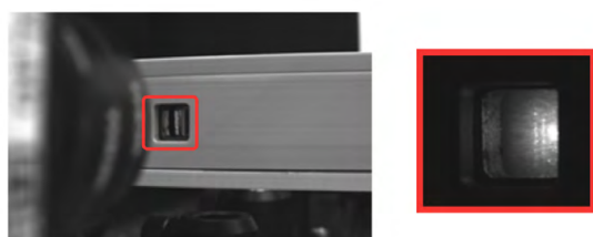
Figure 25.9: Heated rubidium vapor cell. Inset: Fluorescence excited by resonant light.
