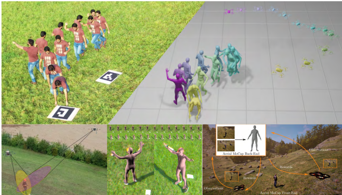
Figure 4.27: Real image sequence (top left). Estimated 3D pose and shape (top right). Two of our MAVs cooperatively detecting and tracking a person on-board in real time (bottom left). Cropped ROIs of images from both MAVs and estimated 3D pose and shape overlaid on images (bottom center). DRL-based aerial mocap (bottom right).
