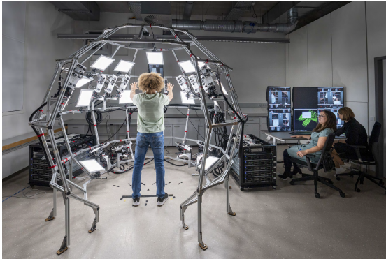
Figure 4.15: Our new 4D hand scanner is operated in collaboration with the Haptic Intelligence department. It is able to capture two hands interacting with objects.
