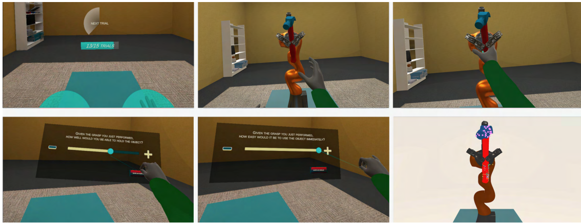
Figure 3.17: Example of a trial in our VR experiment. A KUKA LBR iiwa robot is offering a hammer to the human participant. Top row, left to right: The participant awaits the start of the trial with their hands in the designated area. Then they approach the object held by the robot and grasp it. For explanation only, we depicted the contact points in cyan a posteriori, i.e., the cyan points were not visible during the actual trial. Bottom row, left to right: After the participant has made contact with the object, they answered two questions. The bottom rightmost picture shows an aggregate of the contact points of multiple participants for this scene. Each participant is coded with one color.
