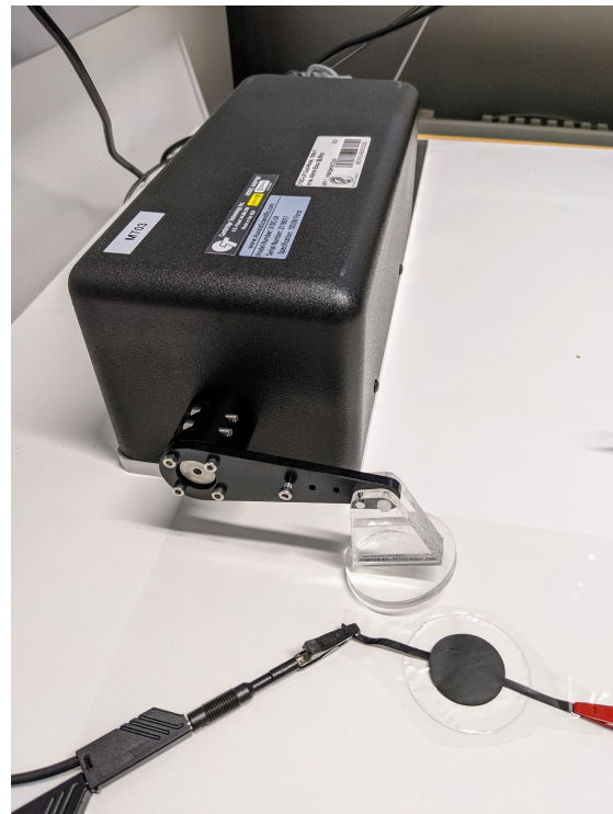
Figure 6.8: Dual-mode muscle tester used for characterization of an electrohydraulic artificial muscle.
