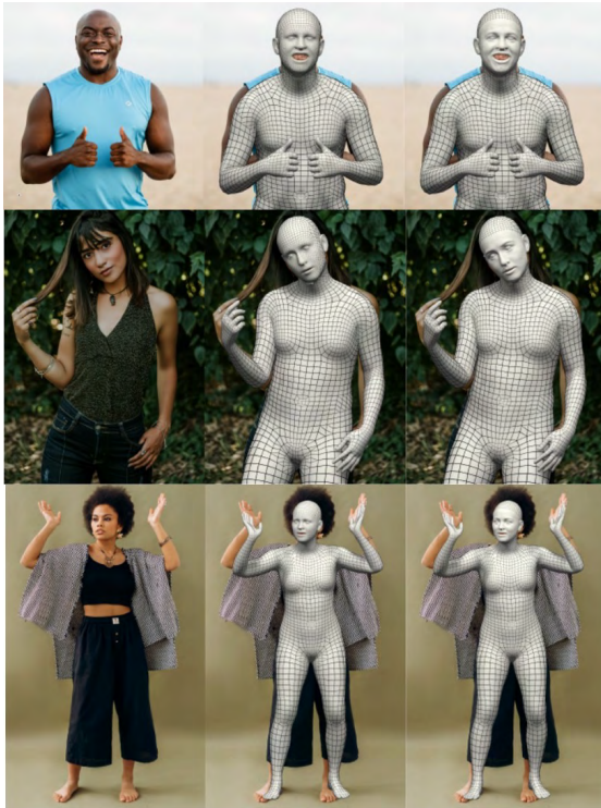
Figure 4.5: Examples of full-body expressive pose and shape estimation with PIXIE. Left to right: Input image, pose and coarse face shape, with detailed face shape. Note how PIXIE is robust to occlusion by the image frame and clothing.
