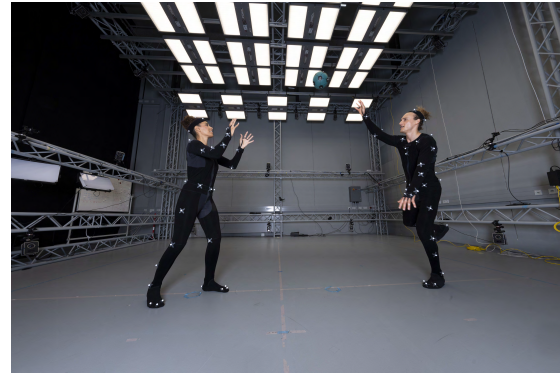
Figure 4.17: Our motion capture space includes a 54-camera Vicon motion capture system a multi-camera video capture system and specially designed lighting system.
