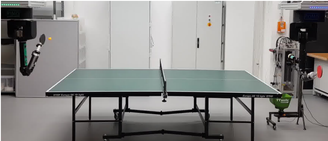
Figure 2.11: We studied a single robot playing table tennis against a human or ball gun in the past. In 2018, we migrated to a new setup with sufficient space for two robots opposing each other. We aim to achieve collaborative table tennis play with the Barrett WAM robot arm and our muscular robots as well as compare performance of motor and muscular actuation using methods from robotic skill learning.
