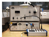
Figure 6.7: High-voltage power amplifier (bottom) and high voltage electrostatic voltmeter (top) for evaluation of electrostatic transducers.
