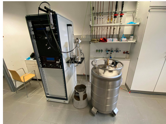
Figure 6.11: Dielectric spectrometer with high voltage controller, alpha-A phase analyzer, and liquid nitrogen tank.
